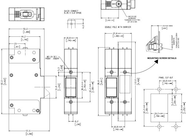
TOLERANCE ± 0.4 UNLESS OTHERWISE SPECIFIED (DIMENSION IN BRACKETS ARE IN INCH)
